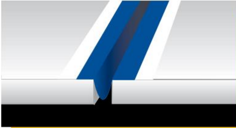
Positioning of Mapeband inside an expansion joint
